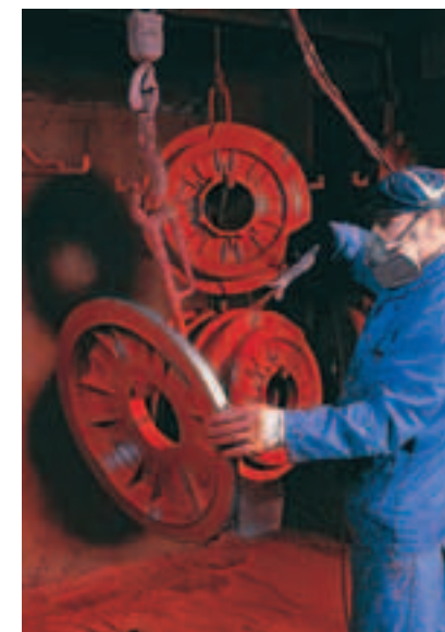
Casted parts get a durable surface by spraying. Componenta Karkkila Oy, Finland
