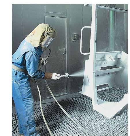
The majority of existing spraying equipment is easily converted to using water-based paints. Application of primer to a Wille s cabin at Vilakone Oy, Finland
