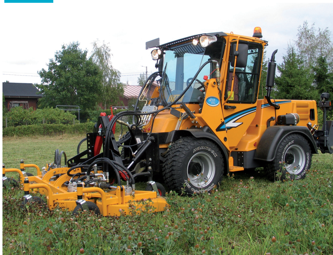
Fonte two-component water-based epoxy primer has very good anticorrosive properties and is resistant to mechanical wear and chemical attack. Wille multi-purpose machine and lawn mower manufactured by Vilakone Oy, Finland, are painted with water-based Fontecryl EP Primer before getting a powder coating finish.
